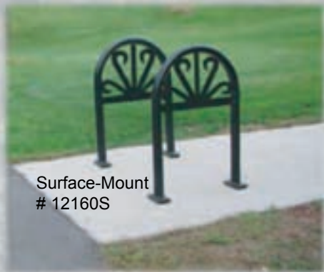
Surface-Mount 3/8" Steel Plate 5/8" Holes 4.5" centers
